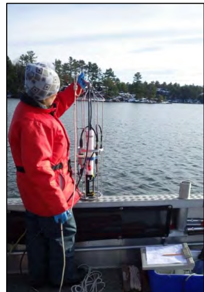
Taking measurements with vertical profiler
